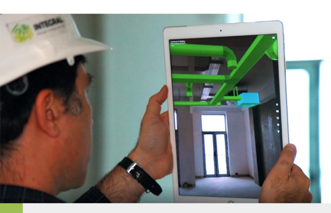
On the design stage team of BIM technicians developed detailed and realistic model of MEP systems taking into consideration project requirements. BIM model used in pre-construction stage and was ready to handover to construction project implementation team. Using application based on augmented reality team of BIM technicians provided ongoing support on construction stage.
